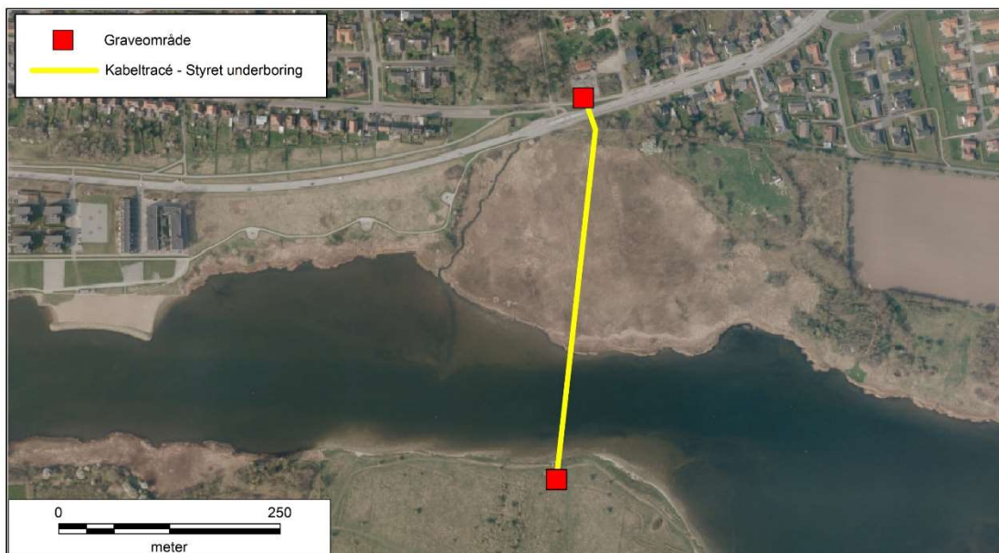
Figur 2 Tracéet for styret underboring under Haderslev Fjord.
