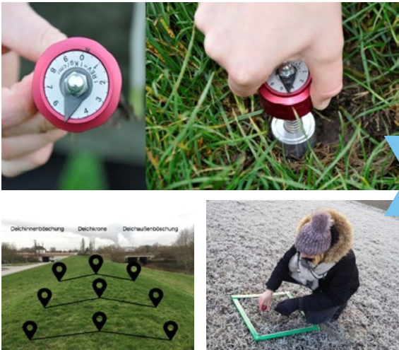
Figure 5.3: Condition assessment: example onsite method to assess the shear stress within a coastal dike as part of the dike inspection procedure
