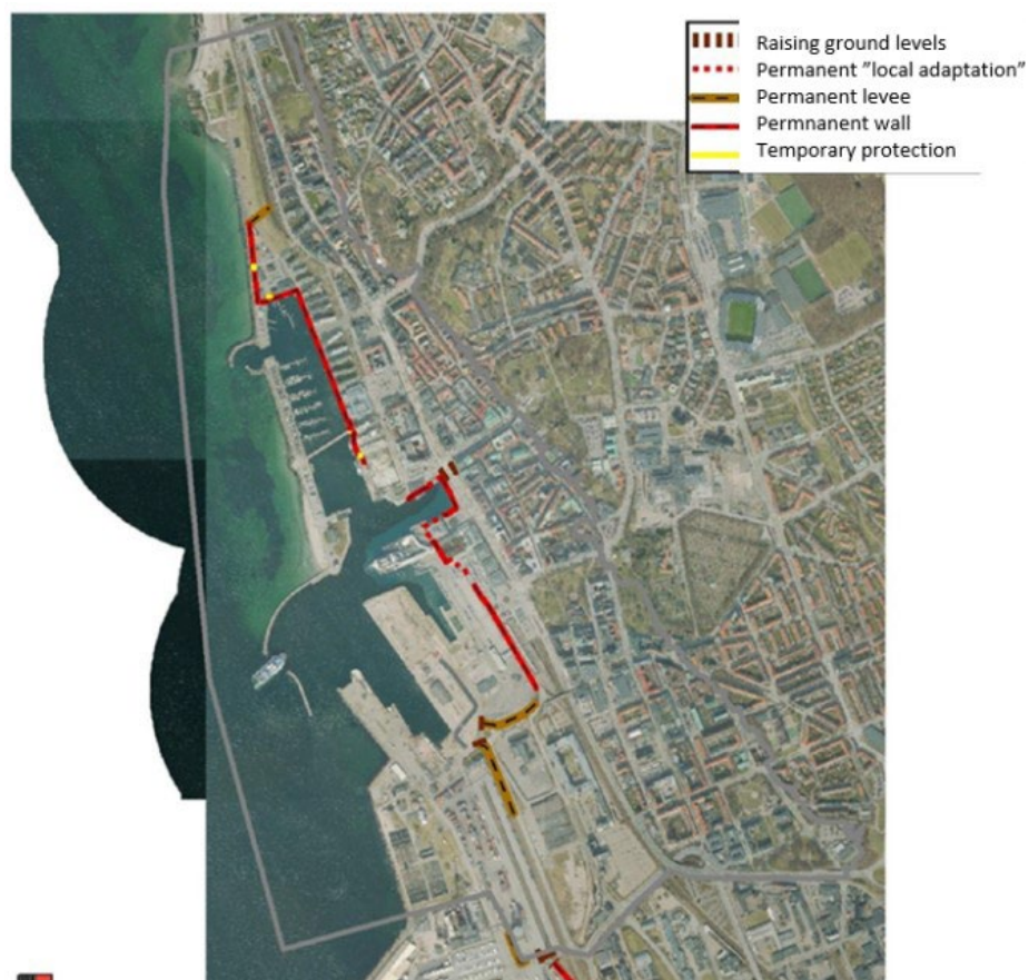
Figure 6. Proposal of inner protection including raising ground levels, permanent local adaptation, permanent levee, permanent wall and temporary protection.
