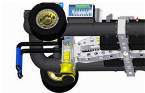
FIGURE 3 FRONT ARM WITH TENSIONER- 500 KG PULL FORCE.
