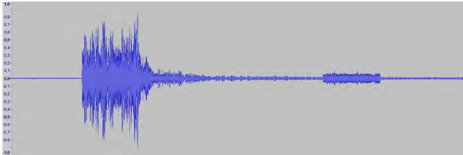
Figure 5.3: Raw data snap shot of recorded pulse at 17:06:17, where the USBL unit pulse is seen on the left hand side, and the transponder response pulse is seen on the right hand side.
