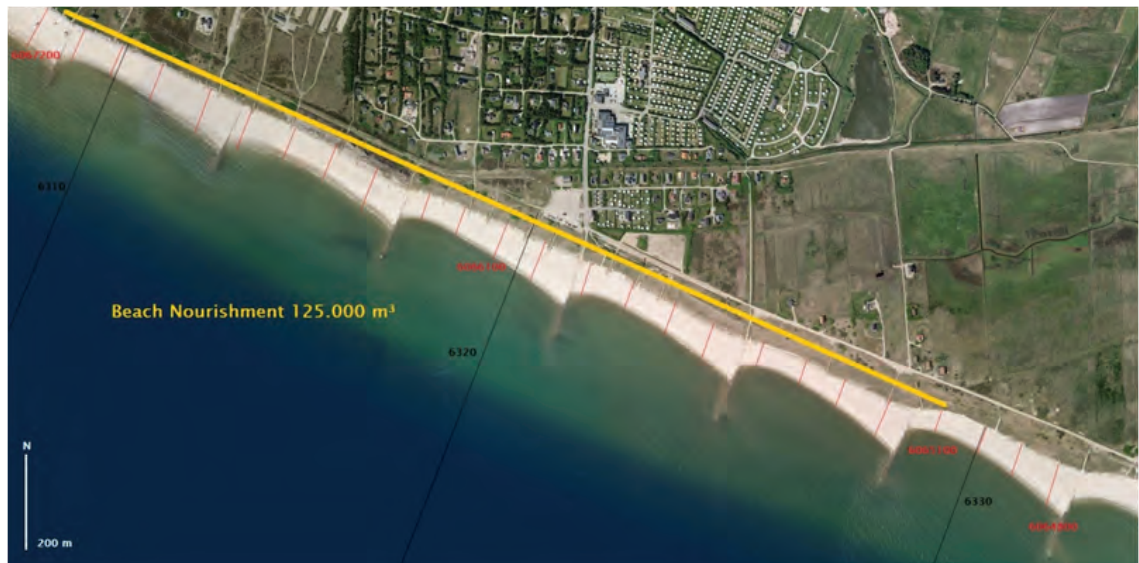
Figure 3.1. Nourishment site with survey lines (red), nourished area (on the beach in length marked by yellow line) and DCA survey lines 6310 - 6330 (black).
